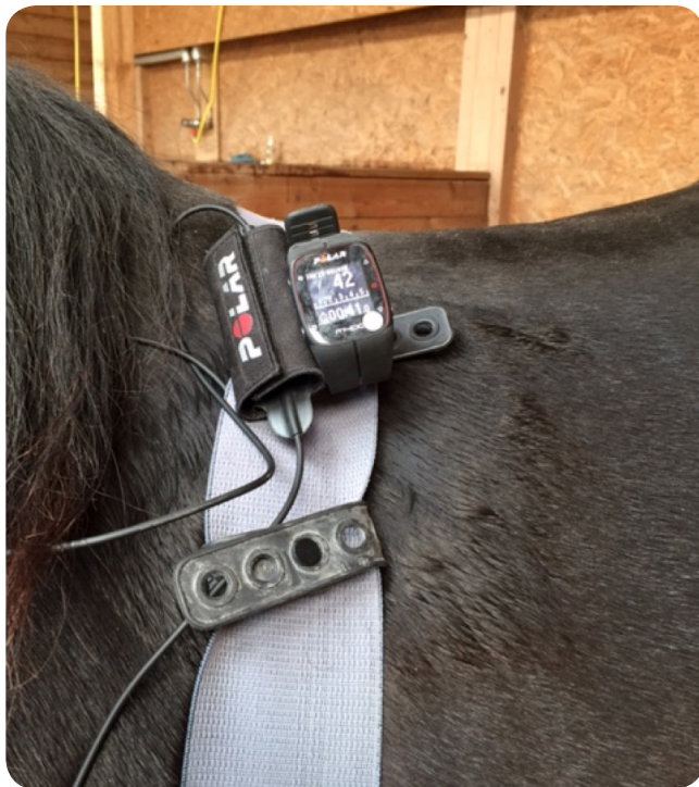
Fig. 2: POLAR equine M400 heart rate recording system fixed to a horse. / POLAR equine M400 Trainingscomputer angebracht an einem Pferd mittels Deckengurt.
